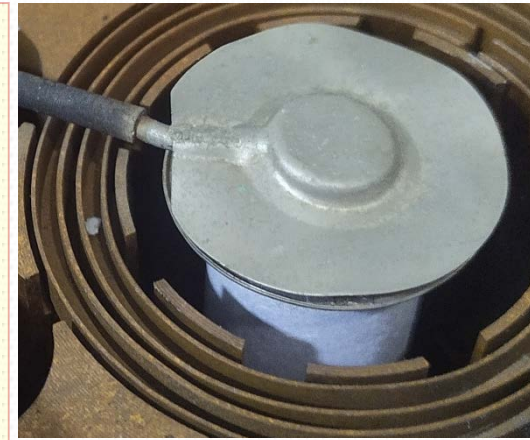
Oxide coated cathode inside Magnetron
