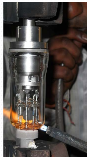
Water-cooled diode during glass blowing
