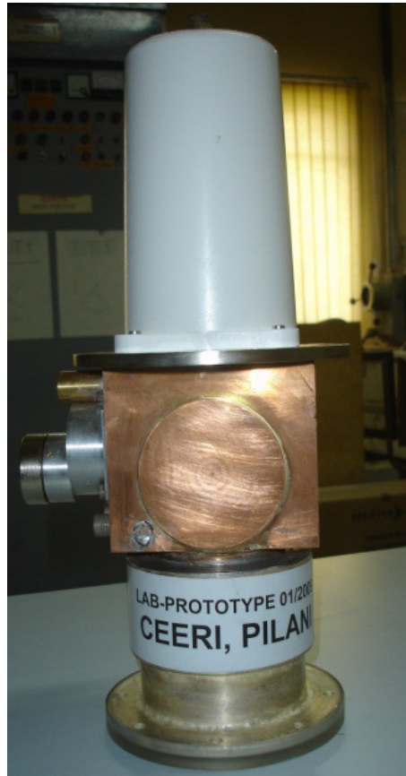
2.6 MW S-Band Magnetron
