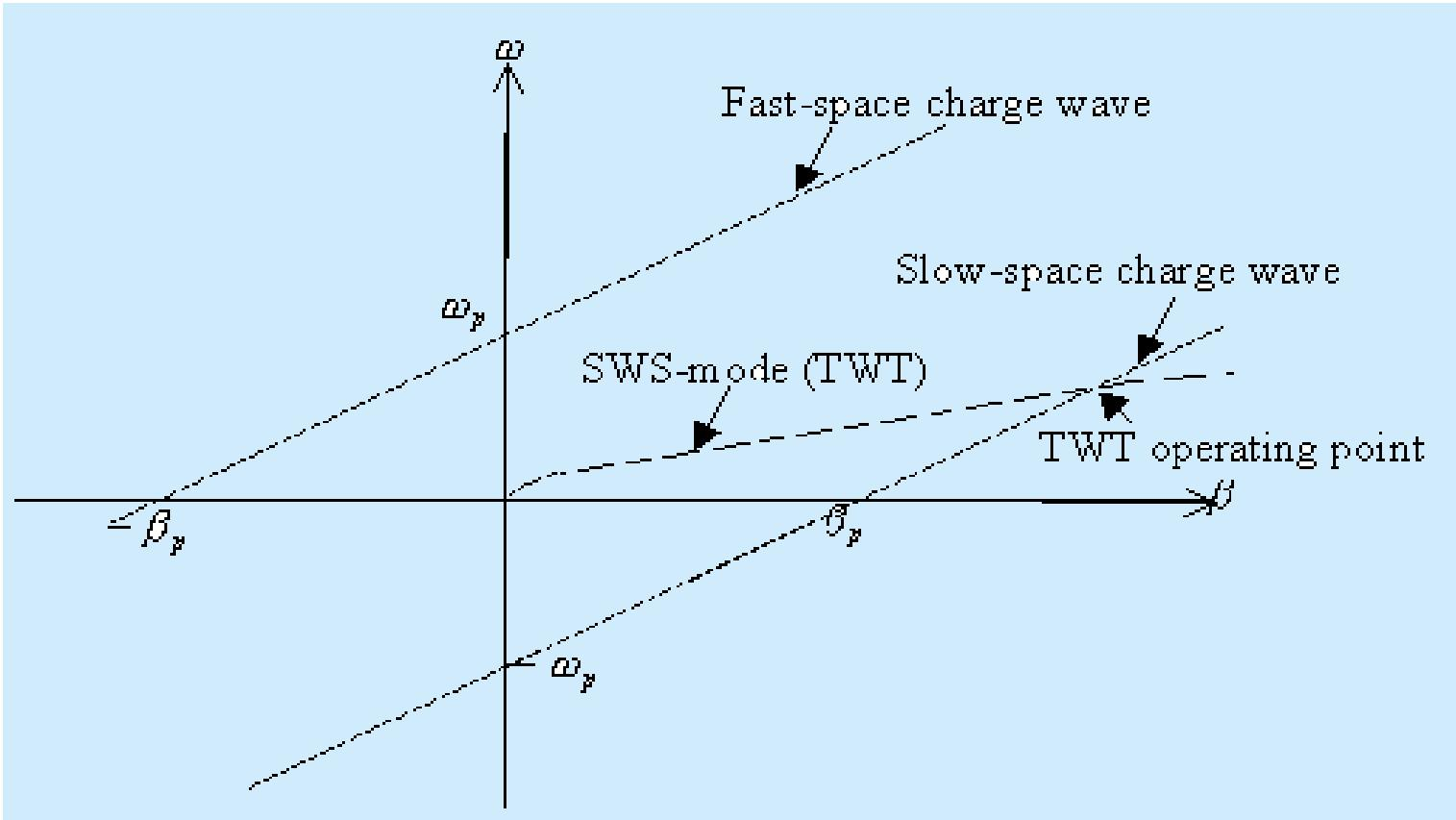
The operating point of the TWT corresponds to the intersection between the  $\omega$  -  $\beta$  dispersion plot of the slow space-charge wave and that of a forward circuit wave.
