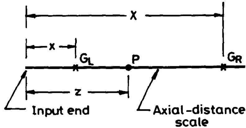
Effect of the element of a modulated beam at a point on the circuit (transmission line) is simulated by an infinitesimal current generator at that point.
