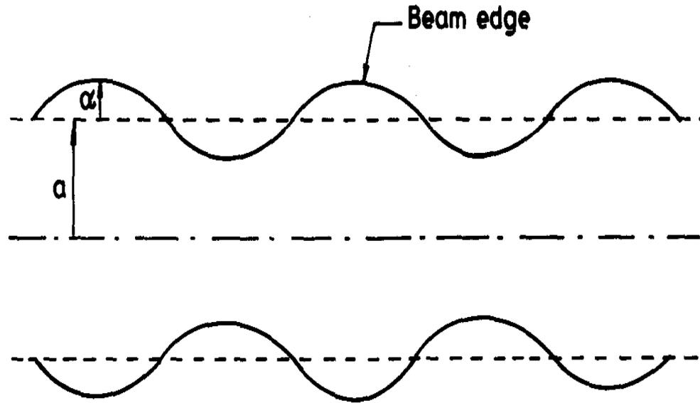
**Beam-scalloping: sinusoidal variation of the beam-edge radius along the structure if the cathode is magnetically shielded ( $B_k = 0$ ) and the beam radius at the entry plane ( $z = 0$ ) is the value that is desired to be maintained constant at  $r = r_M = a$ . Here,  $\alpha$  is the maximum value of the radius variation  $\delta$ .**
