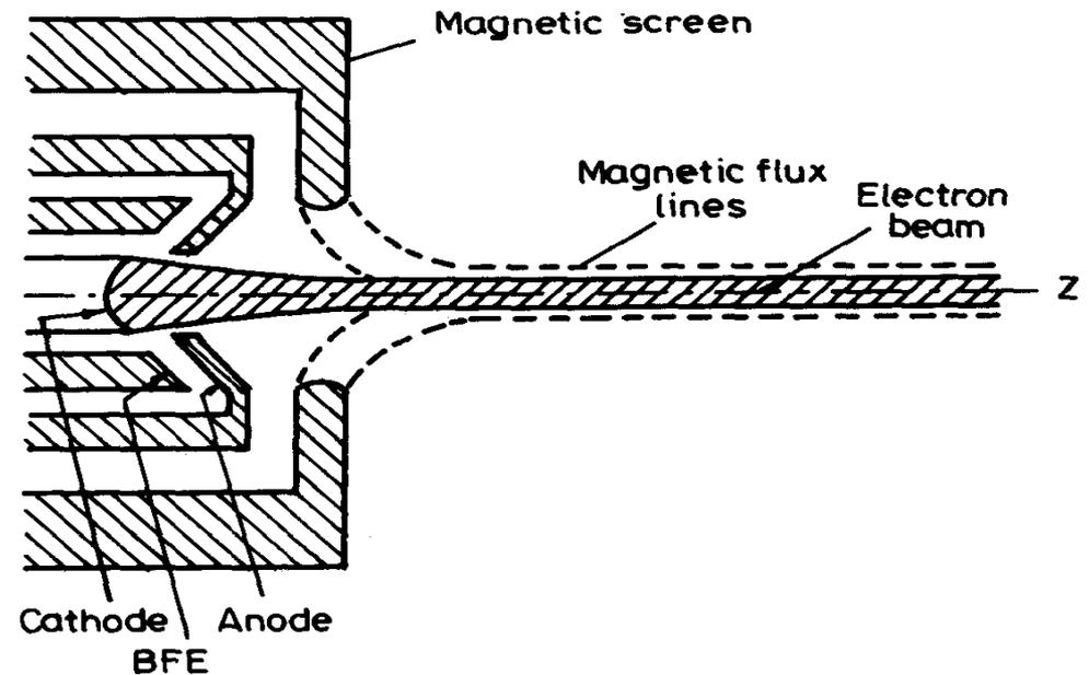
**Schematic representation of Brillouin focusing showing a magnetically shielded cathode**
