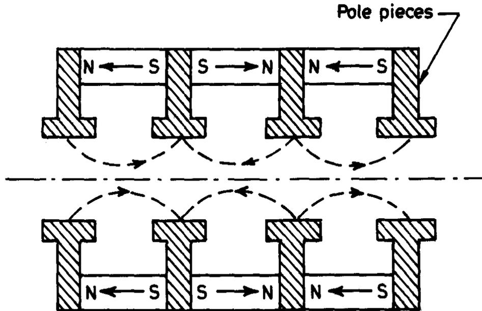
A typical arrangement of magnetic pole pieces between magnets to bring magnetic flux density close to the axis of an axially magnetized PPM.
