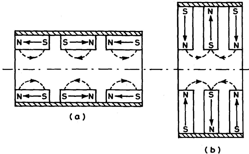
Ring-magnet cells (shown typically, three, in number) in a PPM for the axial (a) and radial magnetization (b) showing magnetic flux lines (dotted) inside the stricture.
