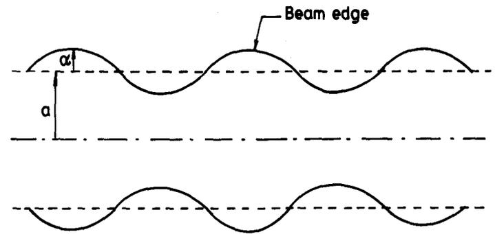
**Beam-scalloping: sinusoidal variation of the beam-edge radius along the structure if the cathode is magnetically shielded ( $B_k = 0$ ) and the beam radius at the entry plane ( $z = 0$ ) has the value that is desired to be maintained constant at  $r = r_M = a$ . Here,  $\alpha$  is the maximum value of the radius variation  $\delta$ .**
