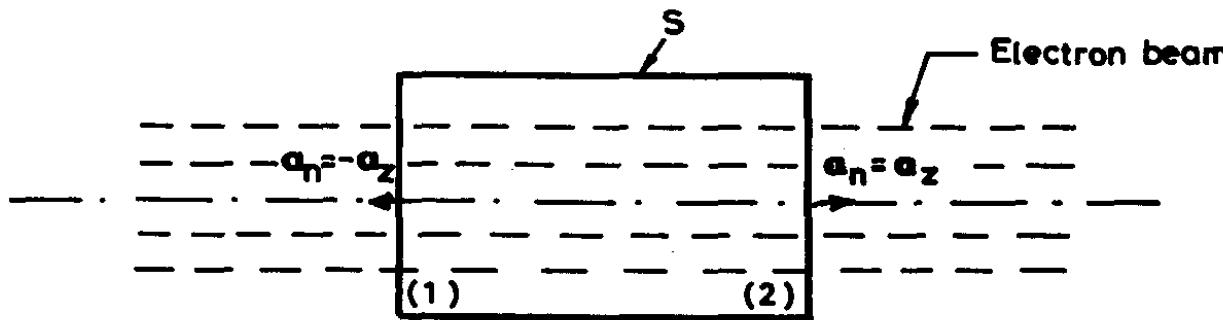
Closed surface (S) of integration enclosing a portion of a linear beam between two reference cross sections 1 and 2.
