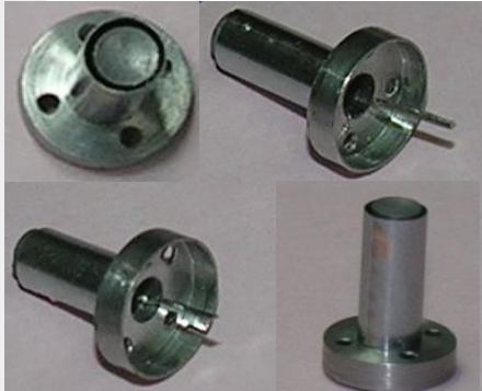
Small \Phi 3.1 mm for TWT, Klystron, J > 50\text{A}/\text{cm}^2
