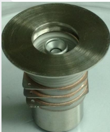
Cathode mounted inside electron gun
