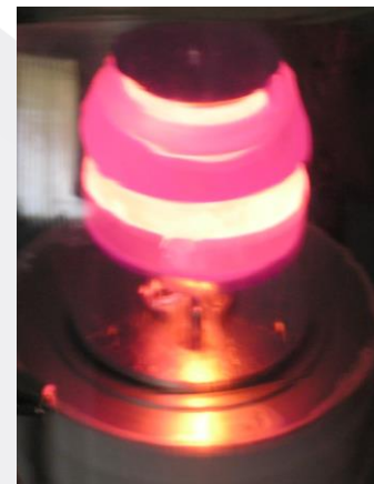
Gyrotron cathode under hot condition
