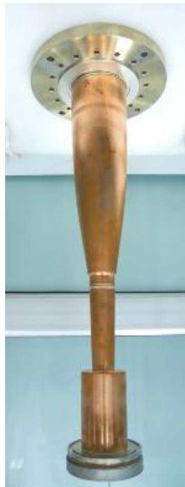
Beam Tunnel + Cavity + NLT + Flange Assembly
