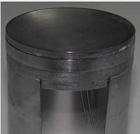
S-Band Klystron cathode \Phi 50 mm diameter
