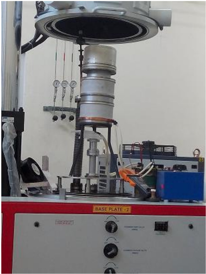
Cathode activation of GCTM
