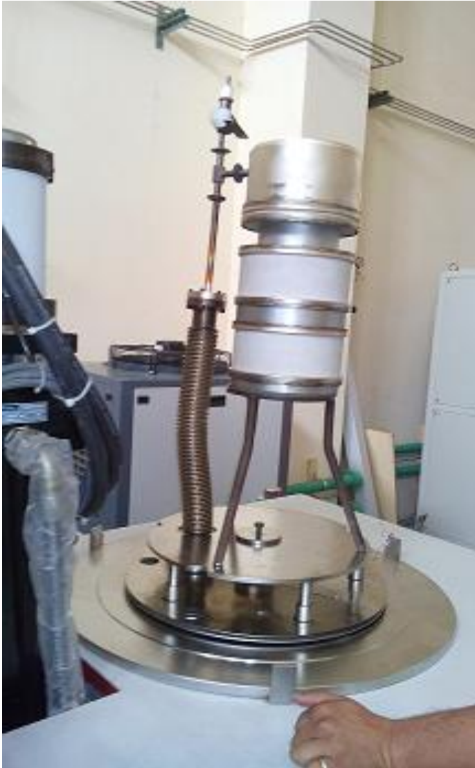
GCTM on vacuum processing station
