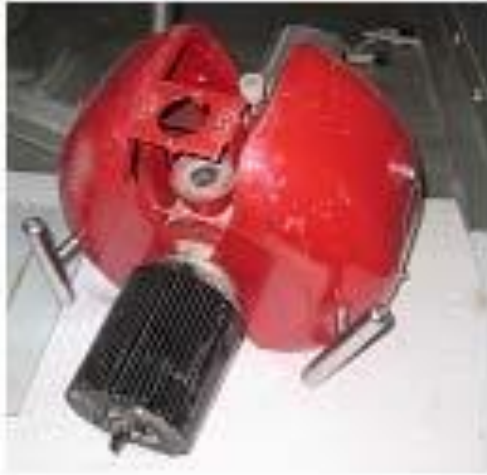
1 kW CW L/S-band Klystron
