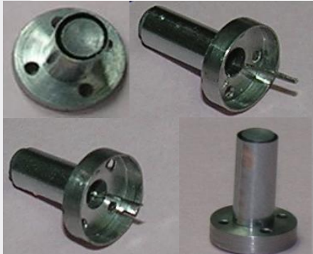
Small \Phi 3.1 mm for TWT, Klystron, J > 50 \text{ A/cm}^2
