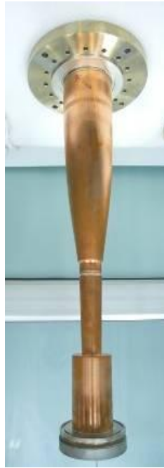
Beam Tunnel + Cavity + NLT + Flange Assembly
