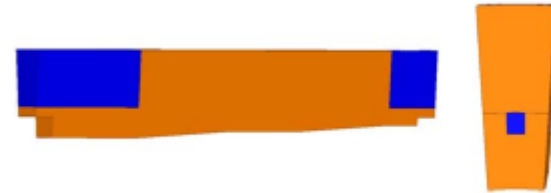
Simulation domain used in the ANSYS with the flow of water (blue region).
