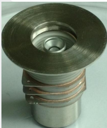
Cathode mounted inside electron gun
