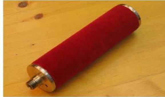
Final part of cathode (diameter 5 cm) out of stainless steel covered with polyester velvet on the essence its length. [5]
