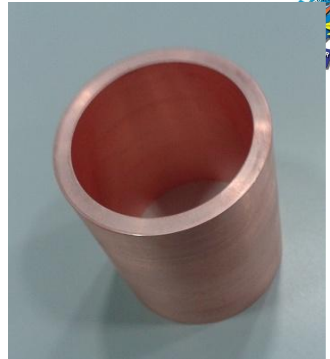
Fig. Fabricated cavity for 170 GHz
