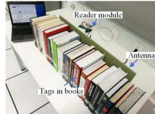
Fig. 15. Test scenario for reader antenna measurements.
