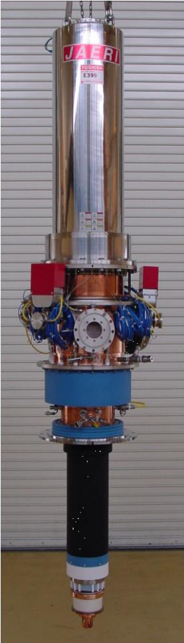
JAERI / TOSHIBA 170 GHz, 0.82 MW (0.6MW) 600s (1h)
