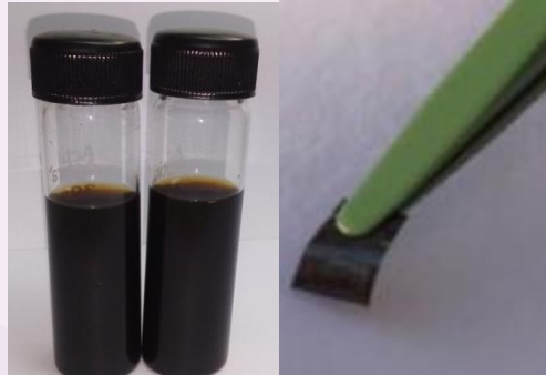
Synthesis of Graphene Oxide using Modified Hummers
